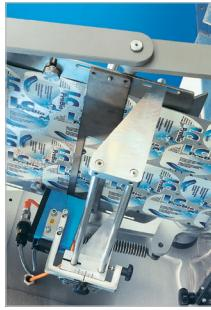
The foil surface can be embossed and coated for easy lid dispensing. The machine is equipped with a table for web splicing.
